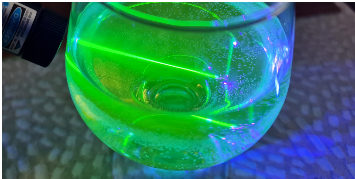
Figure 4: Extremely strong fluorescence of a disodium fluorescein solution under violet laser illumination. The original beam is visible only in reflected light. Weak fluorescence of textile in transmitted light is caused by optical brighteners in laundry detergent.
