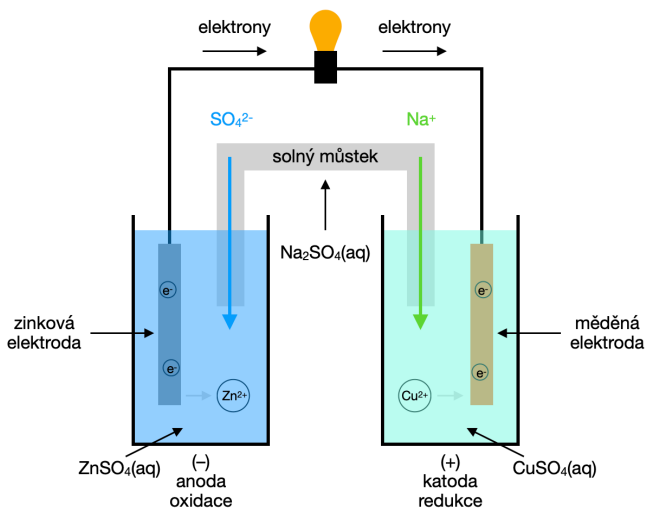
Figure 1: A recall of Daniell cell, which was introduced in the first episode of the series.
