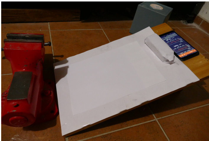
Figure 1: Photo of experiment setup. A sheet of office paper on an inclined plane, the head of a hammer wrapped in paper, and a mobile phone. Rigid object in the back – flower pot.
