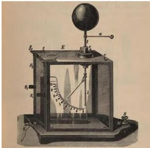
Figure 1: Kolbe's electrometer – the hand of the device is deflected by electrostatic interaction<sup>1</sup>
