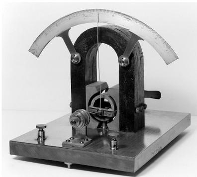
Figure 6: D'Arsonval galvanometer<sup>9</sup>
