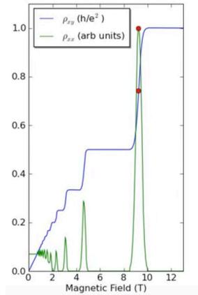
Figure 10: The dependence of resistance on magnetic flux density<sup>14</sup>
