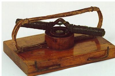
Figure 4: Jedlik's electric motor<sup>6</sup>
