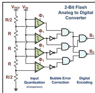
Figure 8: Diagram of flash ADC converter<sup>11</sup>
