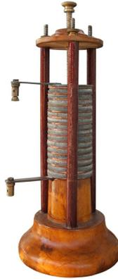
Figure 2: Voltaic pile – source of constant DC voltage<sup>3</sup>
