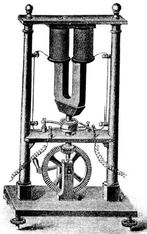
Figure 3: Hippolyte Pixii's dynamo – the U-shaped magnet is turned by a crank under a pair of coils<sup>5</sup>
