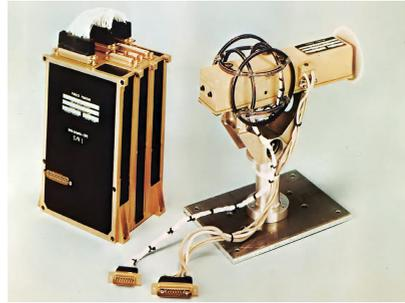
Figure 12: Magnetometer used in the Pioneer 10 and 11 probes<sup>16</sup>
