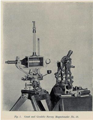
Figure 11: Land surveying magnetometer<sup>15</sup>
