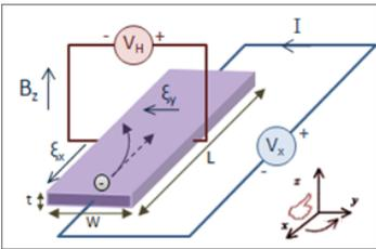
Figure 9: The geometry of the Hall effect<sup>13</sup>
