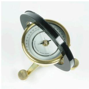
Figure 5: Tangent galvanometer<sup>8</sup>
