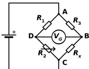
Figure 7: Diagram of the Wheatstone Bridge<sup>10</sup>
